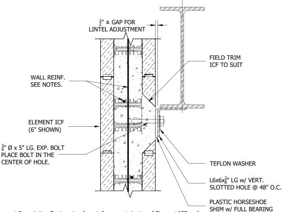
Refer to the Element Prescriptive Engineering for reinforcement design of Element ICF walls.
