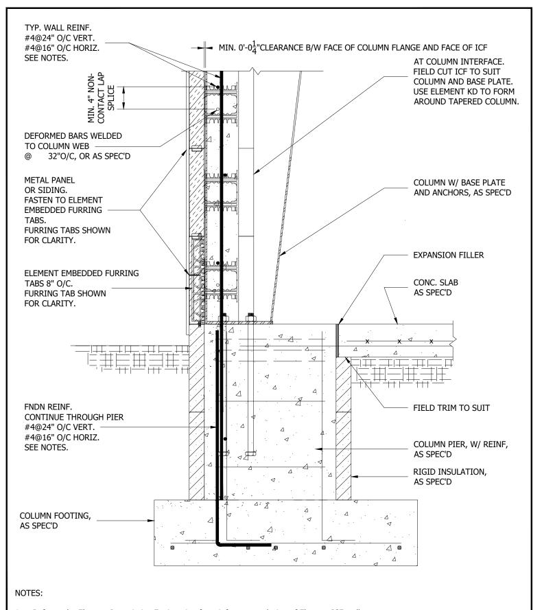
Refer to the Element Prescriptive Engineering for reinforcement design of Element ICF walls.
