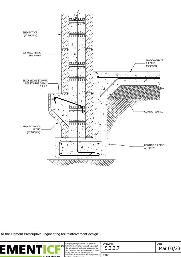
THICKENED SLAB INTEGRATED WITH **ELEMENT BRICK LEDGE**
