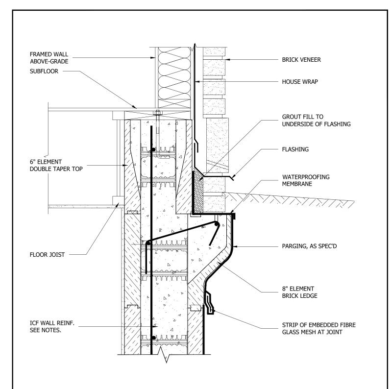
Element Prescriptive Engineering for reinforcement design of Element ICF walls. Element Brick Ledge Stirrup detail drawings for stirrup dimensions.
