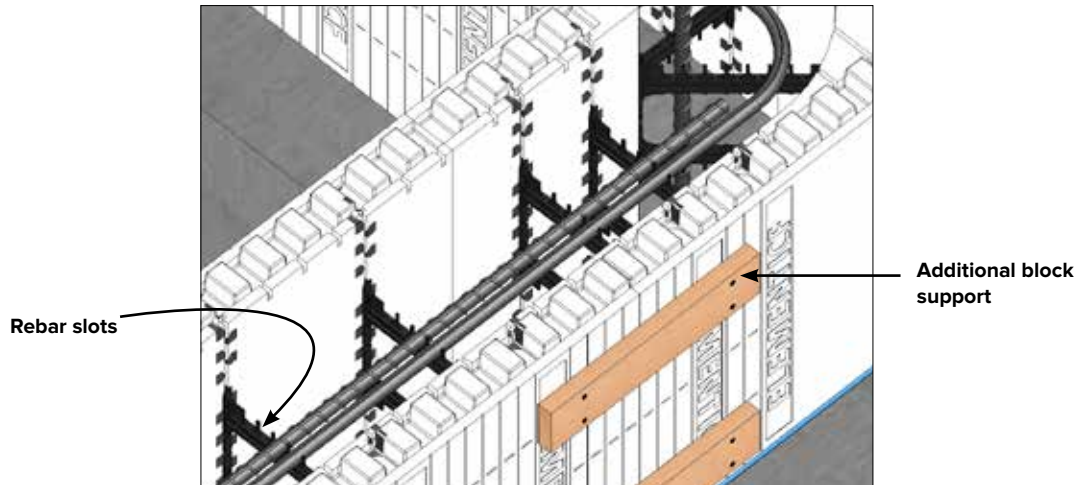
Place reinforcement and necessary additional block support prior to installing the second course.
