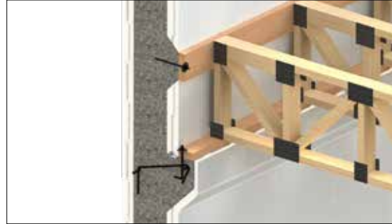
Top chord bearing on Element Brick Ledge.
