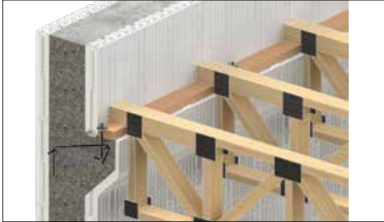
Top chord bearing on Element Brick Ledge.
