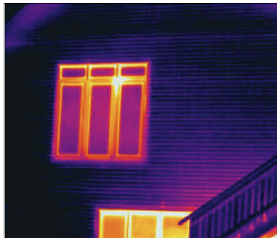
Thermal image of exterior ICF wall showing no heat escape through the wall. Continuous thick insulation with a solid concrete core wall prevents thermal bridging and heat escape through Element walls.
